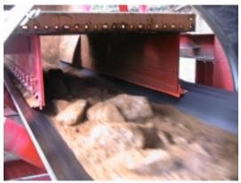
Figure 23 – Material on the receiving conveyor coming right out of one of the transfer stations.
