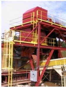
Figure 24 - Splitter/Tripper discharge area on the overland conveyor system of the 72-inch wide belt.
